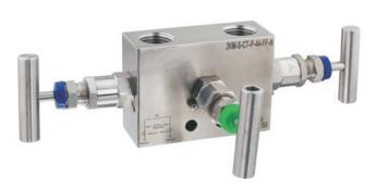
With threaded vertical port inlets and outlets. The isolating bonnets are positioned on the left and right hand side and the equalizing bonnet is positioned on the front. This manifold is specially designed as miniature valve to be remote mounted.
